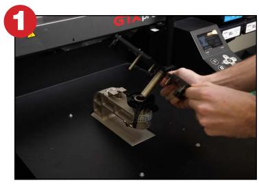
**Step 1:**Insert the T-Lock Base into the platen stem of the Brother DTG printer.
