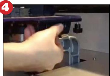
**Step 4:**Secure the T-Lock Wrap Around Insert by rotating the center piece in the T-Lock brackets.
